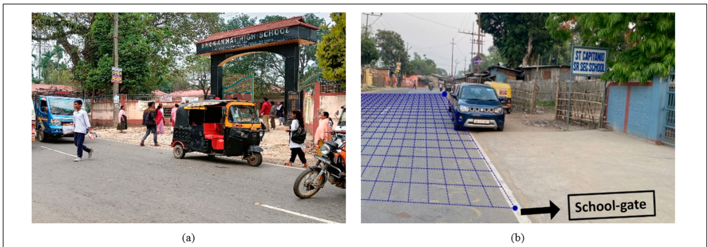
Figure 4. a) Photograph of a site used in case study and b) layout of virtual gridlines within the trap length for the extraction of LP data.
